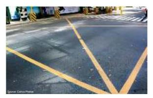
**DO NOT BLOCK INTERSECTION** – lines that form a yellow box within the intersection and yellow diagonal lines forming an "X" inside the box. No vehicle should stay inside the box to avoid obstruction to other motorists
