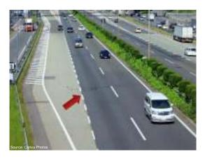
6. TRANSITION LINES – guide the traffic safely to pass obstructions on roadways such as islands, median strips, bridge piers or indicate changes in the width of the traveled portion of the roadway and an increase or reduction in traffic lanes
